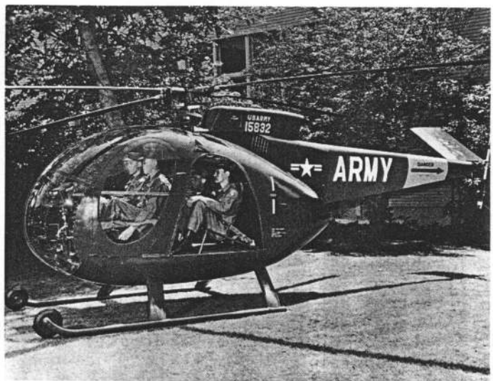
NEW HUGHES MODEL 369 (ARMY DESIGNATION HO-6) HELICOPTER. PHOTO SHOWS HELICOPTER WITHOUT REAR DOOR INSTALLED.
